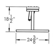
INSTALLATION INSTRUCTIONS: USING THE LUMBER CONNECTION HARDWARE ASSEMBLE THE SEAT TO THE FRAMES (4 CONNECTIONS). ASSEMBLE THE CROSS BRACES TO THE SEAT BRACKETS USING THE LUMBER CONNECTION HARDWARE (2 CONNECTIONS). ASSEMBLE THE FRAMES TO THE CROSS BRACES USING THE METAL CONNECTION HARDWARE 14 CONNECTIONS).
