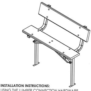
USING THE LUMBER CONNECTION HARDWARE ASSEMBLE THE SEAT AND BACK REST TO THE FRAMES (8 CONNECTIONS). ASSEMBLE THE CROSS BRACES TO THE SEAT BRACKETS USING THE LUMBER CONNECTION HARDWARE (2 CONNECTIONS). ASSEMBLE THE FRAMES TO THE CROSS BRACES USING THE METAL CONNECTION HARDWARE (4) CONNECTIONS).
